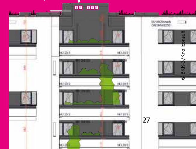
Integration of bat nesting boxes („F“) on building site 10 (Hochh(in)aus, Wiener Heim)
